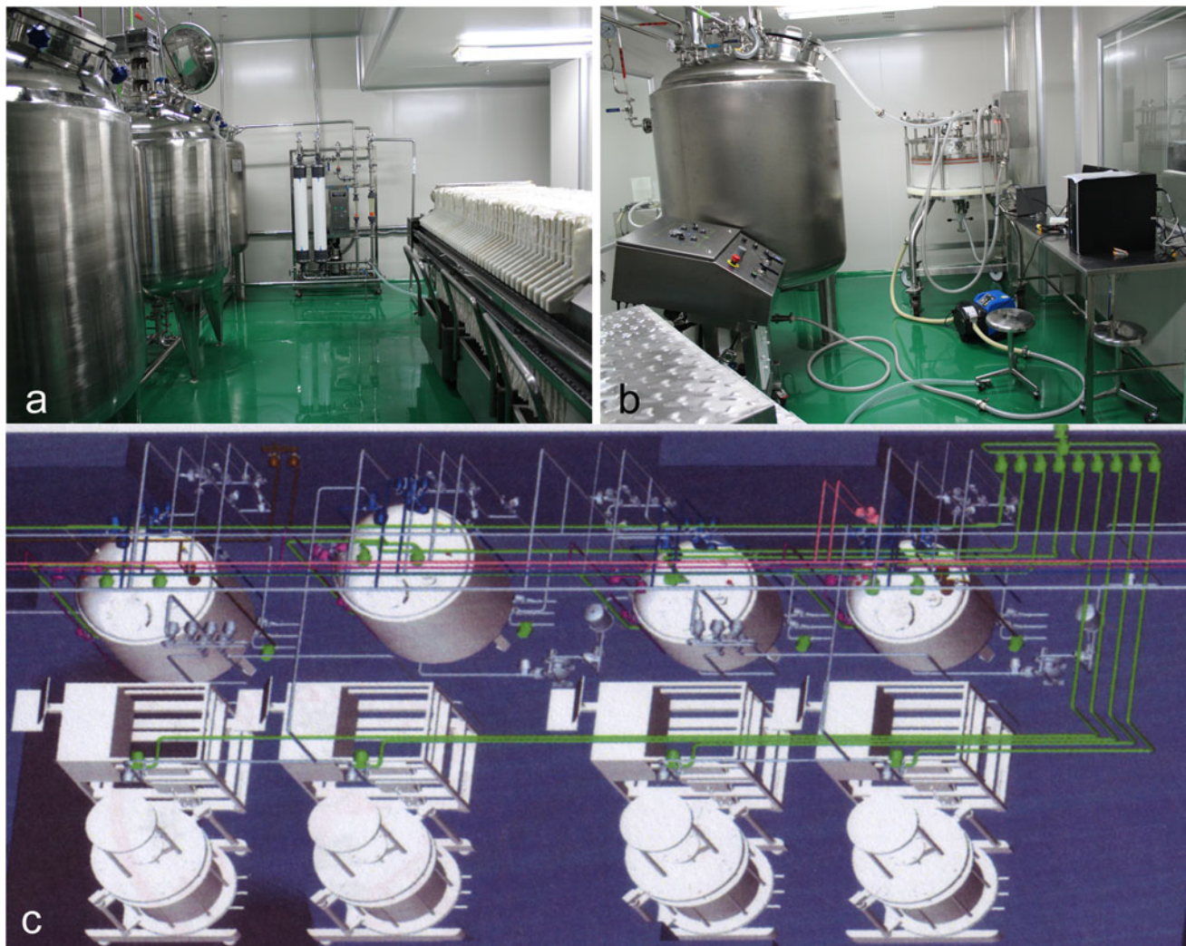
Fig. 6 Pilot facility and large scale manufacturing of OsrHSA from transgenic rice grain. a, b The processing of transgenic rice and purification of OsrHSA as pilot scale; c purification facility for manufacturing of OsrHSA
